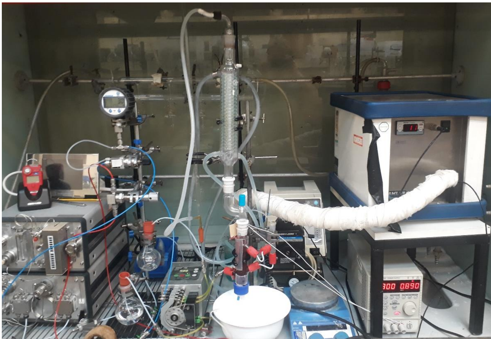
Figure 5-9. Slurry-Bubble Column Reactor set-up in continuous operation
