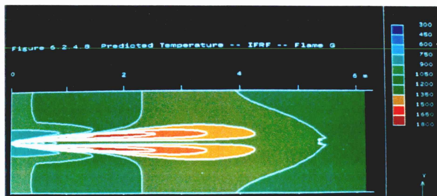
Figure 6.2.4.8 Predicted Temperature - IFRF - Flame G
