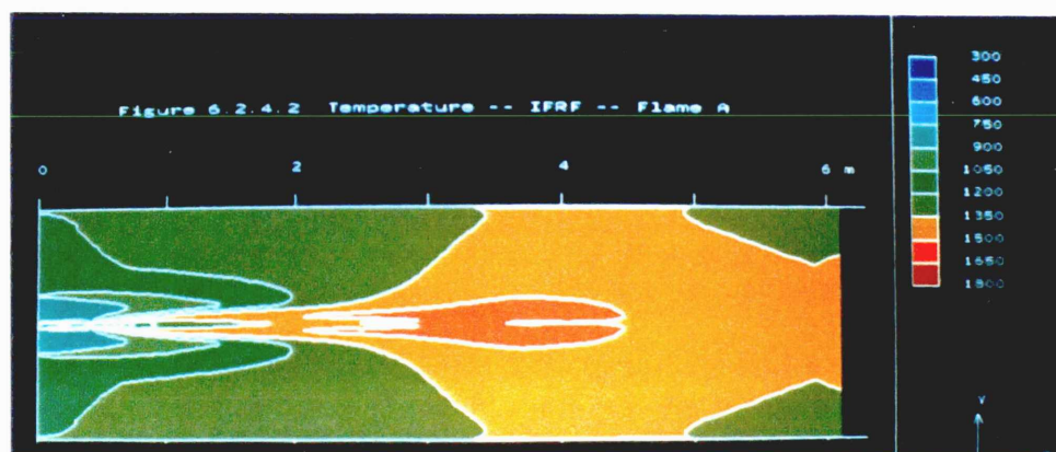
Figure 6.2.4.2 Predicted Temperature - IFRF - Flame A
