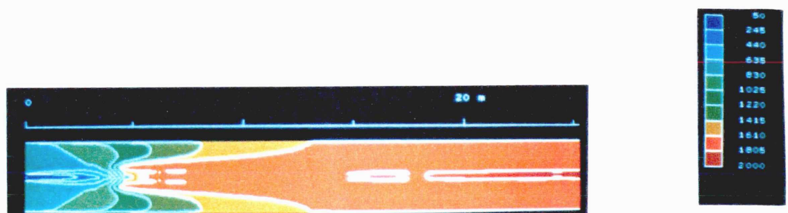
Figure 6.3.2 Temperature for Full Size Cement Kiln Prediction -- Flame MINI
