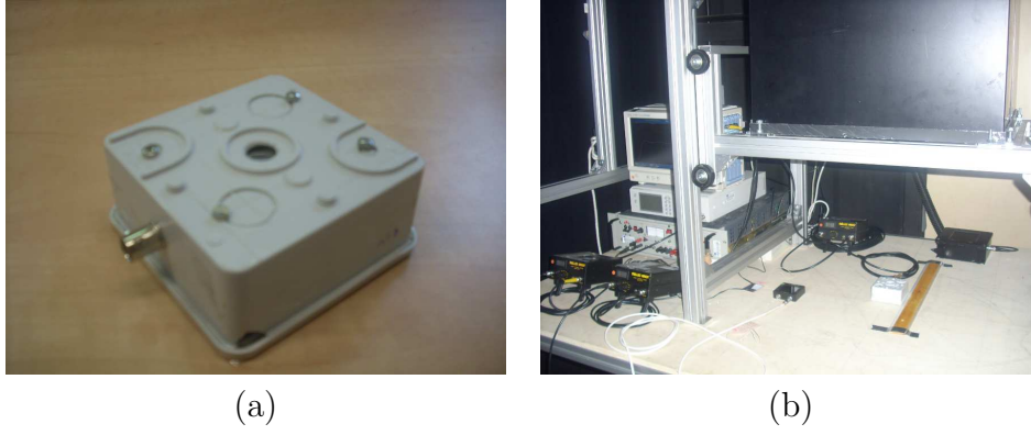
Figure 3.10: Spatial uniformity. (a) c-Si photodiode used as detector (active area: 2.5 \text{ mm}^2 ); (b) measurement setup. The detector has been covered with an OD = 3 neutral density filter for measurements at high intensity.
