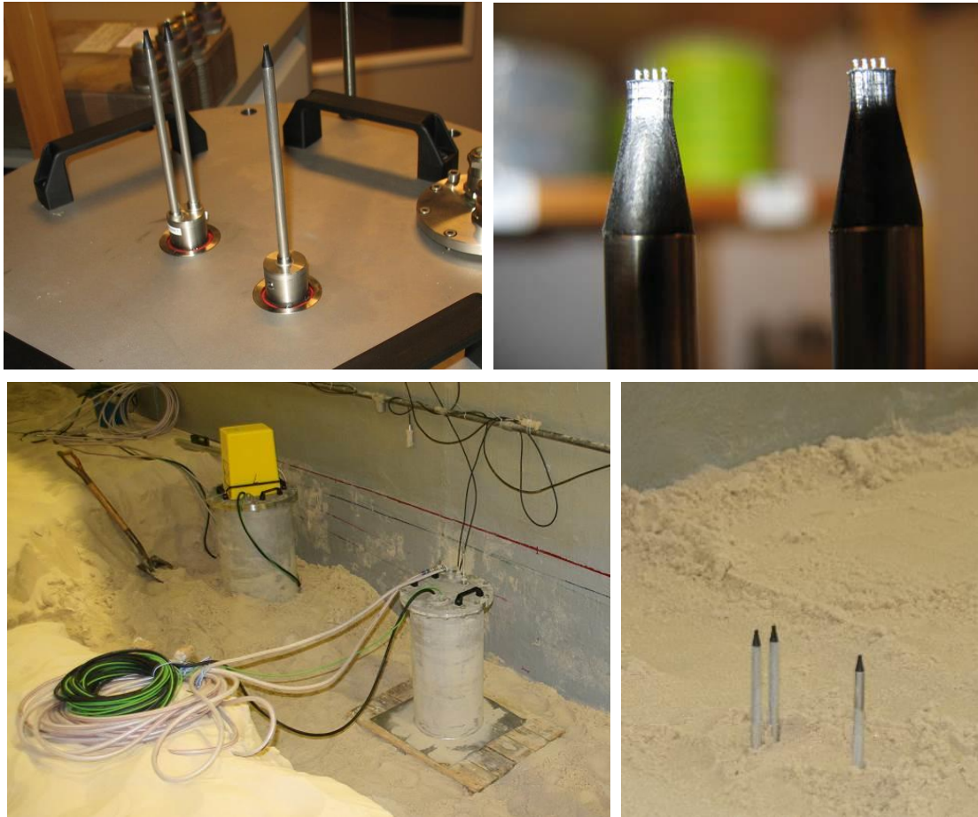
Figure 2. Photos of CCM + system. Top: probes in lowest position (left) and probe sensors (right). Bottom: installation of tanks during an experiment (left) and zoom of probes after installation (right; note that during an experiment, the probes are lowered such that only the probe sensors emerge from the bed).
