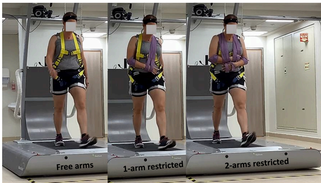
Figure 1. Experimental set-up. Participants walked on a computerized treadmill system with a horizontal movable platform (Balance Tutor, MediTouch Ltd, Tnuvot, Israel) at their preferred walking speed. Participants walked under three conditions, each lasting 120 s, in the following order: (i) unrestricted upper-body movement, ‘free arms’ condition (left); (ii) the dominant arm restricted with a sling, ‘1-arm restricted’ condition (centre); (iii) both arms restricted with slings, ‘2-arms restricted’ condition (right).
