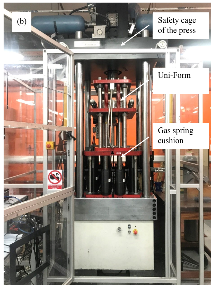
Fig 3.11 Uni-Form installed on the gas spring cushion system in the press
