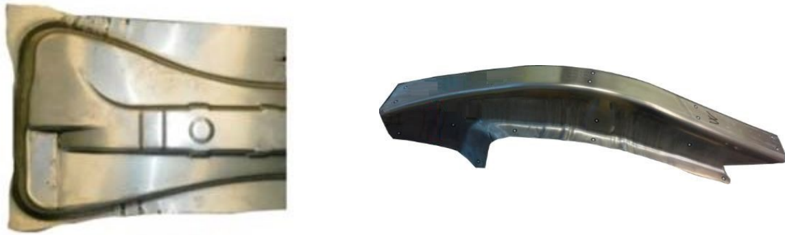
Fig 2.20 W-Temper formed vehicle B-pillar (left) (Sáenz de Argandoña et al., 2015) and Front side member of Volkswagen Touran (right) (Mendiguren et al., 2016)
