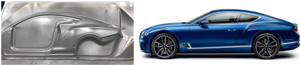
Fig 2.18 Superplastic formed body side panel (left) of BENTLEY Continental GT (right) (Rösner-Kuhn, 2018)
