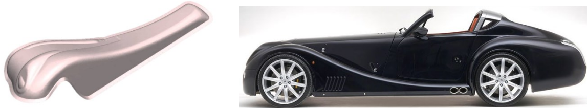
Fig 2.17 Superplastic formed front fender (left) of Morgan AeroMax (right) (Grimes, 2011)
