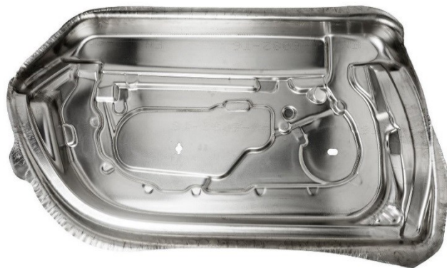
Fig 2.13 HFQ formed door inner of LOTUS concept car (Politis et al., 2013)
