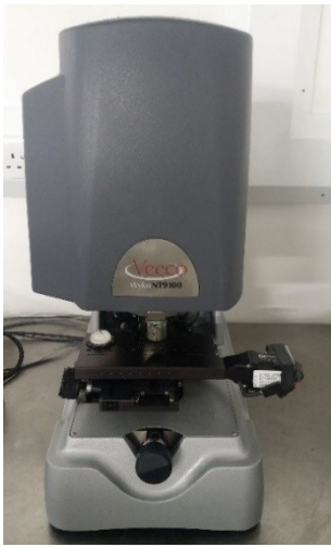
Fig 6.6 Wyko NT9100 Optical Profiling System
