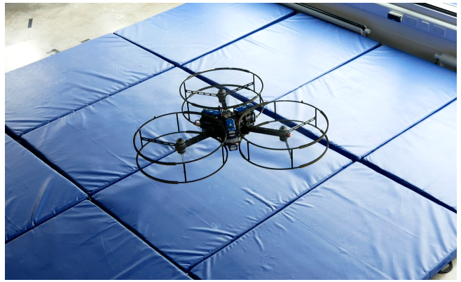
Fig. 3: Flight testing of the platform in the motion tracking arena with a 12.45 kg take-off mass.
