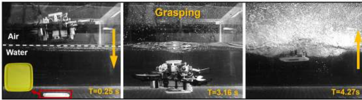
Fig. S20. High-speed images of the robot (with a biomimetic disc mounted underneath) transiting into water, grasping an object, and removing the object from the water.
