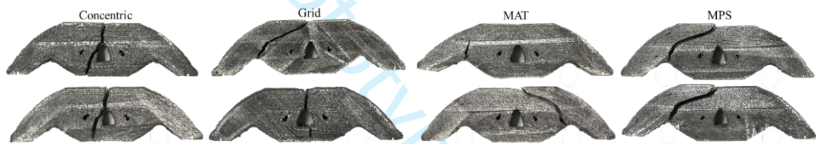
Fig. 16: Macroscopic fractography of the TO-3PB specimens
