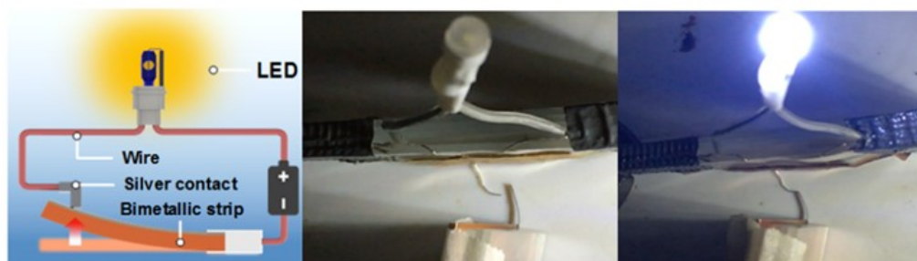
Figure 5.14 Schematic and photos of a simple electrical circuit actuated by the printed bimetallic strip.
