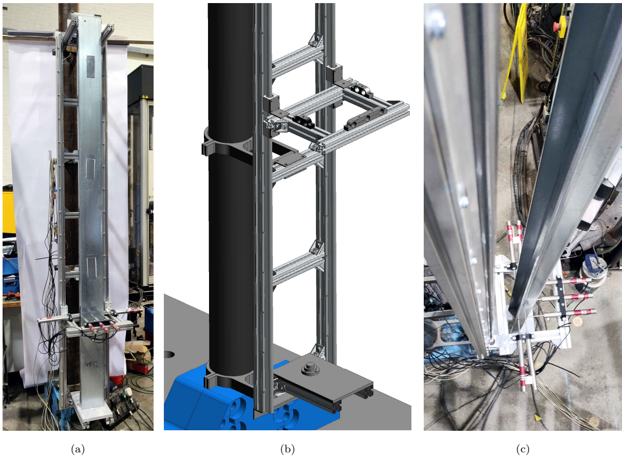
Figure 8: Imperfection rig (a) elevation view (b) schematic and (c) detail of the rails and the LVDTs around the cross-section
