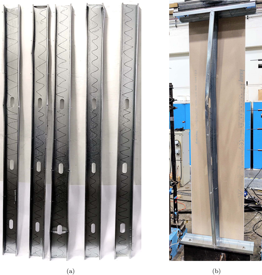
Figure 26: (a) Failure modes of columns sheathed with plasterboard and tested under compression (from left to right – connectors spaced at 600 mm, 300 mm (2 repeated), 150 mm and 75 mm), (b) test specimen with 600 mm connector spacings, post failure (with the sheathing removed to observe the failure mode)
