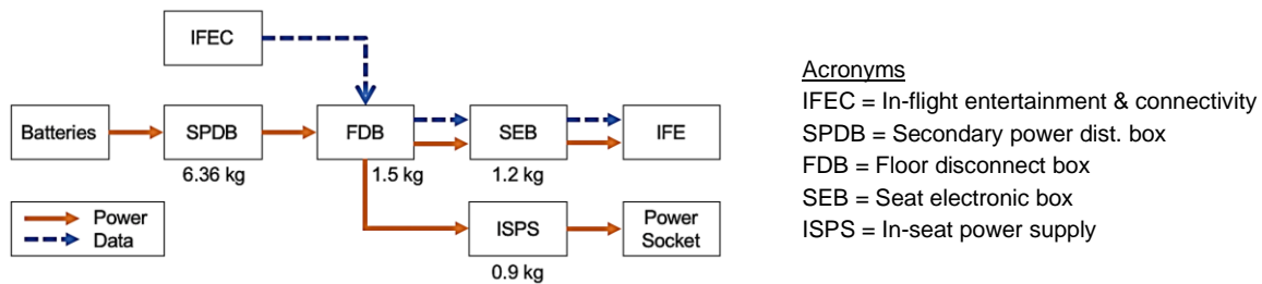
Fig. 2 The power and data connectivity for a conventional in-flight entertainment system.
