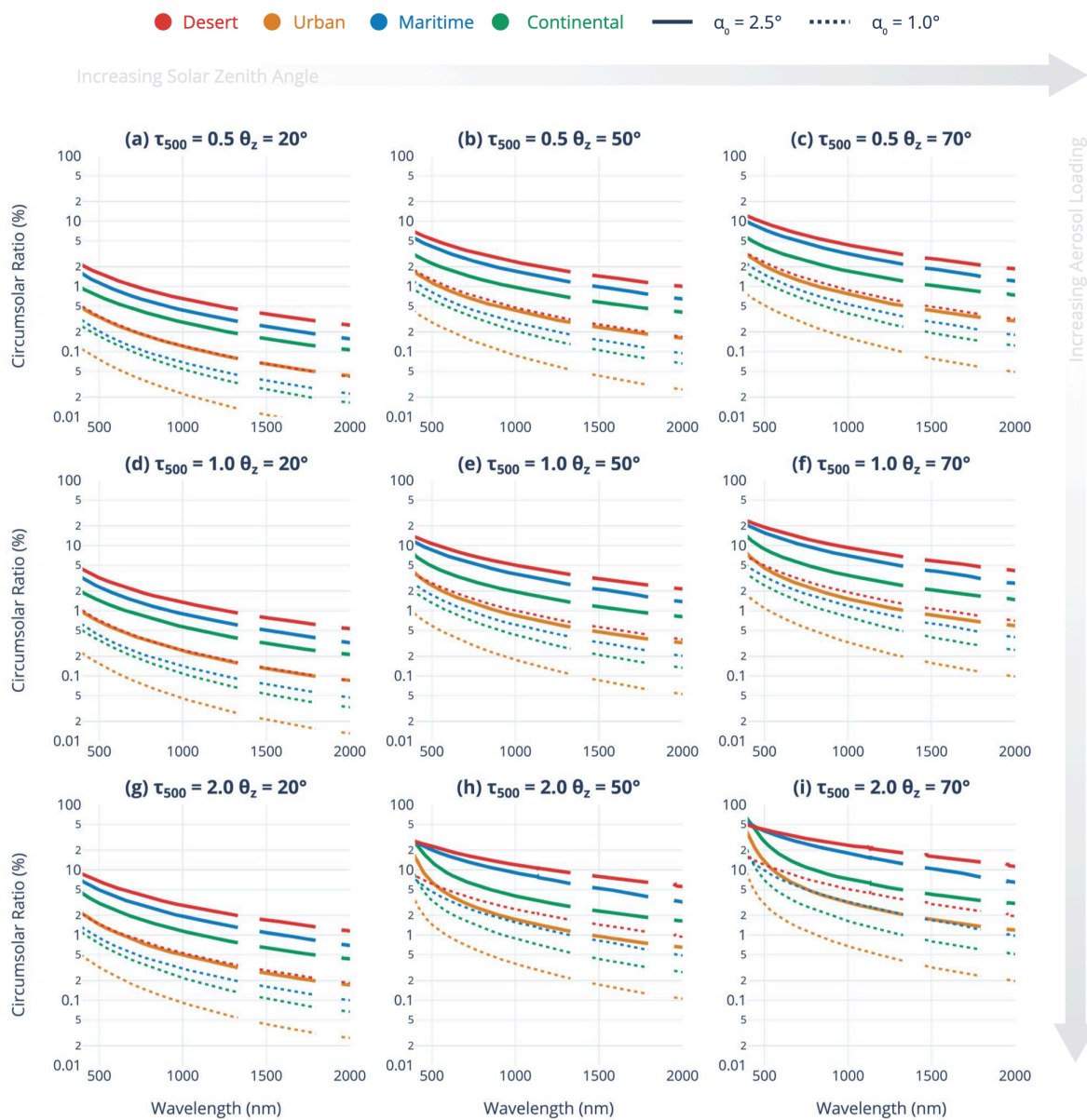
Figure 7: Comparison of CSR_\lambda for selected OPAC aerosol types under various combinations of \theta_z and \tau_\lambda . Regions of substantial water vapour bands are masked out as CSR_\lambda is undefined. Calculations assuming an aperture half angle of 2.5^\circ , typical of pyrhemeters, are shown with solid lines. Calculations assuming an aperture half angle of 1.0^\circ , typical of MJ CPV systems, are shown with dotted lines.
