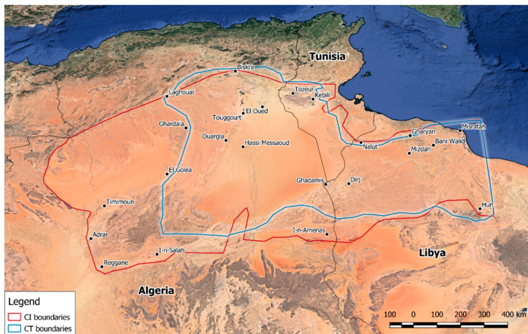
Figure 2. The boundaries of the NWSAS showing the extension of the Continental Intercalary (CI) and the Complex Terminal (CT) aquifers.
