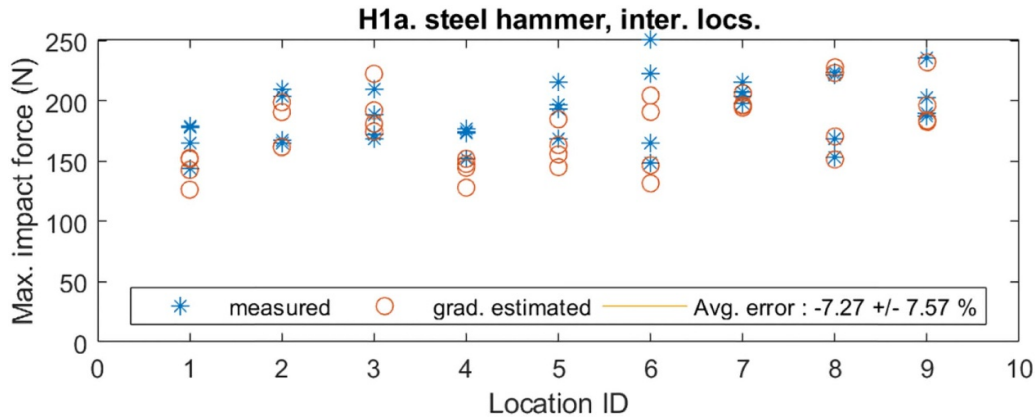
Figure 14. Maximum impact force estimation using gradient method with FMA signal amplitude for the steel hammer at intermediate locations (case H1a).
