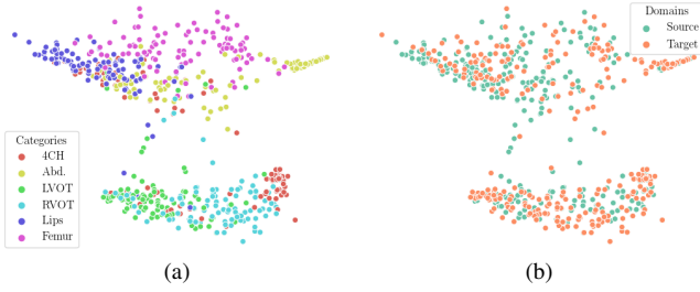
Fig. 6: Feature visualization of MIDNet with t-SNE. We plot categorical features from both domains. (a) The color represents categories. (b) The color represents domains. We observe that the categorical features are domain-invariant and enable the anatomical classification.
