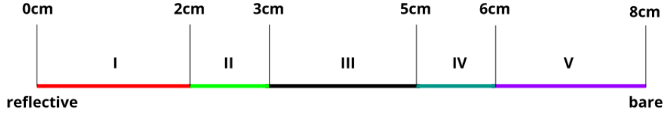
Figure 17: Geometry and boundary conditions for the one dimensional Reed cell 1D radiation shielding verification benchmark test case.
