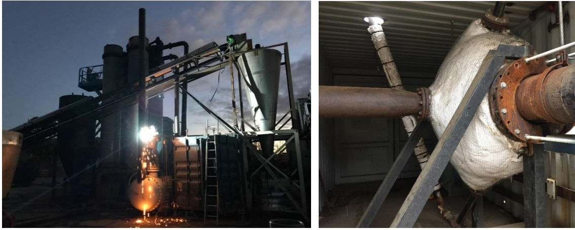
Figure 5. An electrically-enhanced shockwave reactor of 10 tonne per hour without feeding system fits into a 20 ft container. Here, the reactor is configured to gasify solid waste for energy generation.
