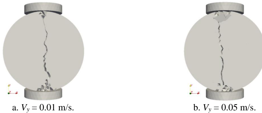
Figure 8: Comparison of final fracture patterns in Brazilian tests obtained from two loading velocities V_y = 0.01 and 0.05 m/s.
