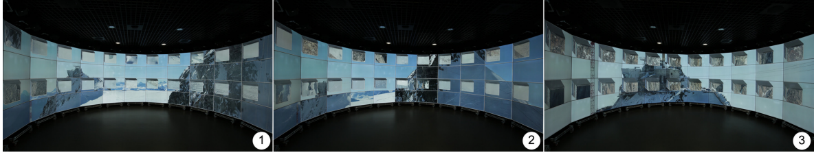
Figure 5: Photographs showing OVE displaying a DZI across many display tiles. These photographs were taken while running T3 and show the DZI displayed across: ①: 416 display tiles with a total resolution of 1.53 gigapixels. ②: 416 display tiles with a total resolution of 6.13 gigapixels. ③: 1000 display tiles with a total resolution of 2.07 gigapixels. Readers may notice a discontinuity between image tiles in photographs ① and ② as the resolution of each tile exceeds that of each individual display making only a portion of each tile visible. This misalignment is more obvious in the videos corresponding to these photographs, which we have provided as supplementary material.
