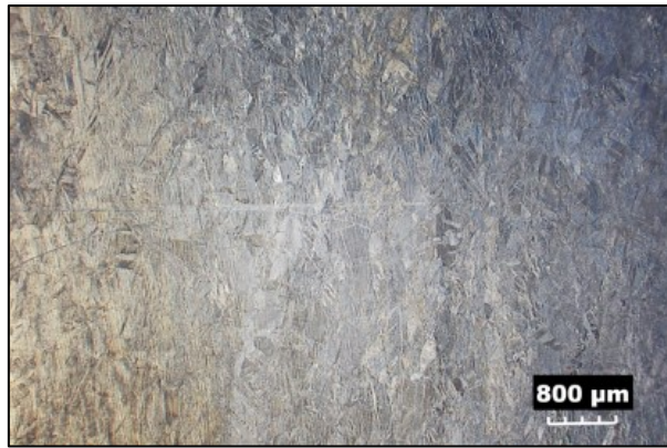
Figure 3.2: Microstructure of a Haynes 25 disc cross section taken using an optical microscope
