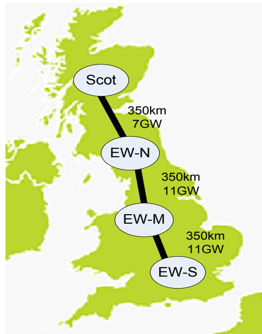
Figure 5.1– Schematic topology and the existing capacity of the GB transmission links between the key regions
