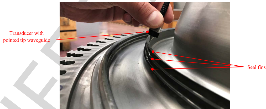
Fig. 10. Photograph showing inspection of a seal fin feature of a jet engine drum.
