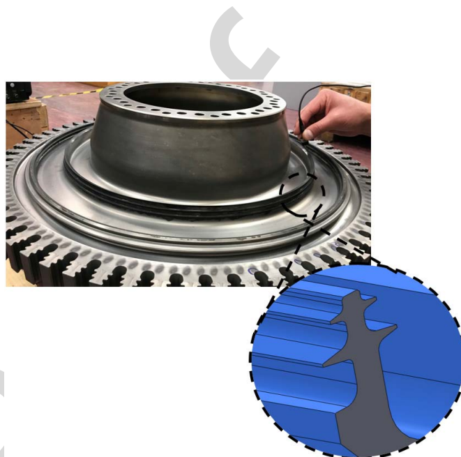
Fig. 1. Photograph of engine drum with inset CAD render of a feature composed of four wedge-like seal fins, the upper two are 2 mm in height and the lower two are 4 mm.
