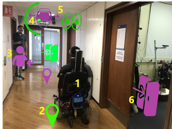
Fig. 1: Composite image of the visualisations rendered on the users view through the AR headset. (1) Smart Wheelchair. (2) We use the marker symbols to represent locations. (3) People - Approach affordances are placed when persons are detected. (4) The cursor and timing bar give feedback to the user during the aiming and selection stages respectively. (5) The different aiming methods available can be selected by the user using an on-board menu. (6) Door - Go Through affordances are shown when open doors are detected. Selected signifiers are shown in green and non-selected signifiers in purple.
