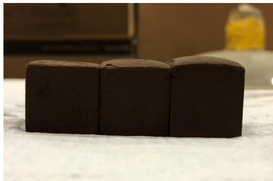
Fig. 6. Photo of lime-FSSA pastes showing slight expansion (10%~30% quicklime from left to right)
