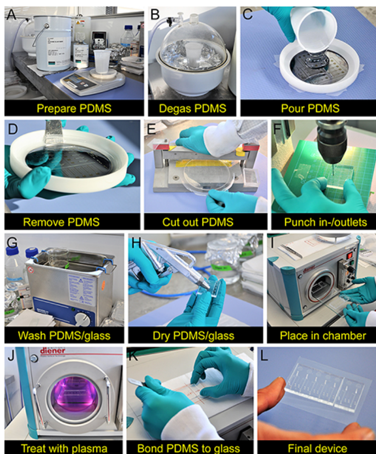
Figure 2. PDMS device fabrication. The processes involved in preparing a PDMS device are illustrated (see Procedure B for detailed information). The PDMS is prepared by mixing the base and curing agent together (A) and degassing the mixture (B). The degassed PDMS is then poured on top of the master mould (C) and then removed after curing in an oven (D). After cutting out (E) and punching holes (F) into the PDMS, it is washed (G), dried (H) and bonded to a glass substrate (I-L). For detailed video instructions on PDMS device fabrication see Video 1.
