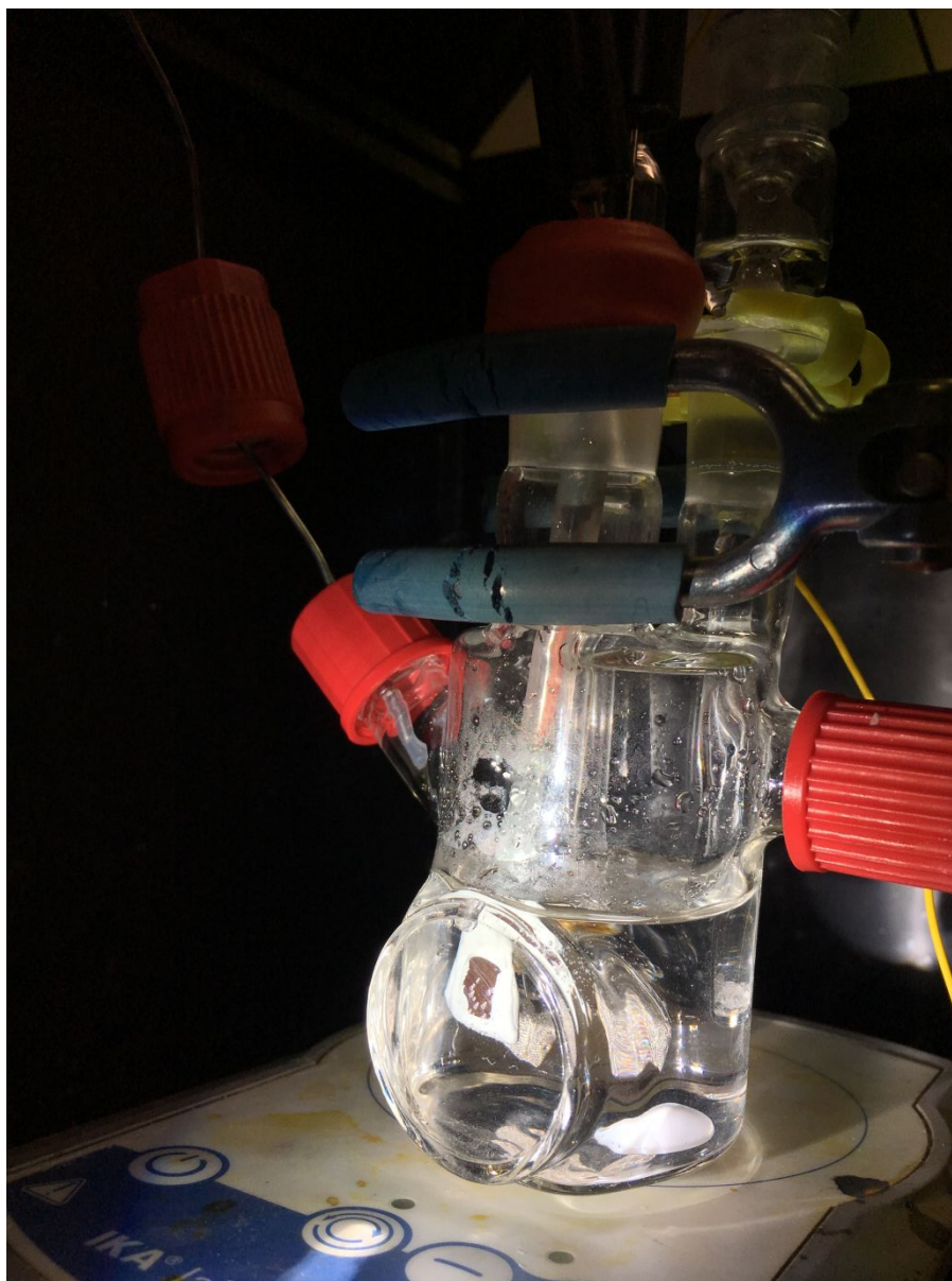
Supplementary Information Figure S11. The experimental setup used for the photoelectrochemical measurements which consists of the working electrode, GaP, Ag/AgCl (sat'd KCl) reference electrode, and a Pt mesh counter electrode immersed in 0.1 M H 2 SO 4 (pH 1.1).
