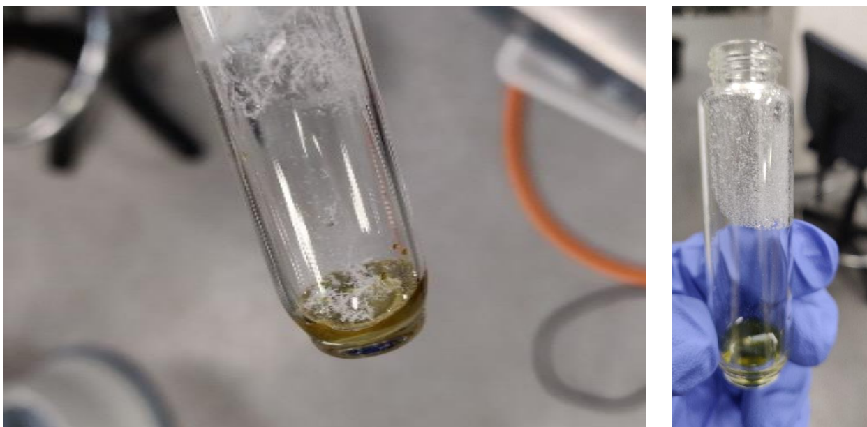
Figure S26. On the left, photograph of the reaction mixture after 6 h showing sublimed DFF (white) while further material precipitates from the reaction mixture. On the right, DFF after vacuum was applied for 6 h at 80 °C.
