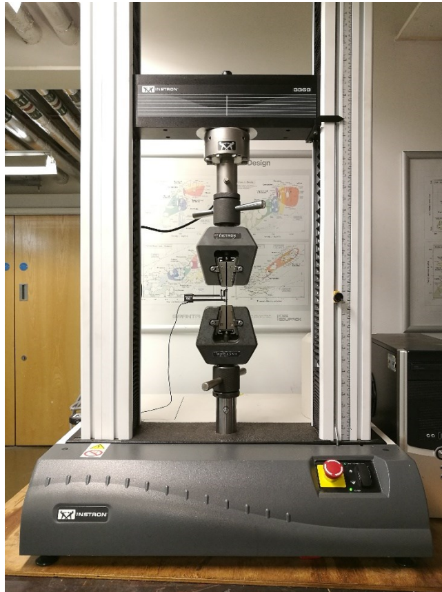
Figure 5.17: Uniaxial tensile tests on a hydraulic Instron machine
