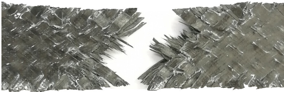
Figure 5.22: Typical failure mode of the CFRP composites after 45° tension
