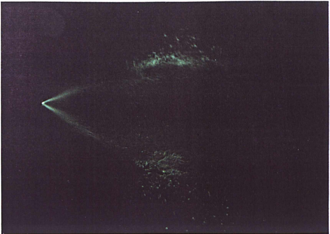
Figure 2.8 Side Cut View of Spray into Swirling Air
