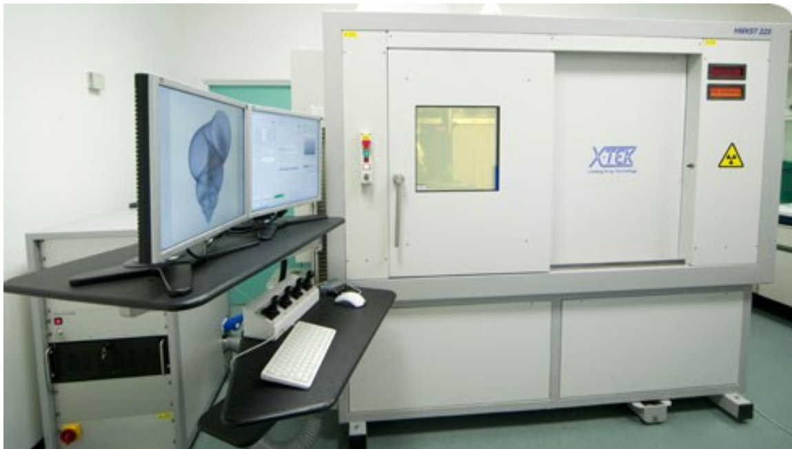
Appendix 3.4 Metris X-Tek HMX ST 225 Micro-CT Scanner at the Imaging and Analysis Centre , London Natural History Museum (image courtesy of Dan Sykes and Farah Ahmed).
