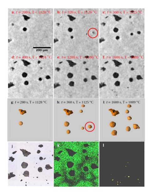
Figure 1: **a-f:** Time series showing 2D sections from tomograms at 6 time instances. Time and average temperature during recording are given in each frame. **g-l:** 3D renderings of selected graphite particles at three time instances corresponding to a-d. **j:** Room temperature microstructure obtained by LOM. **k & l:** EDS maps of silicon and magnesium respectively.
