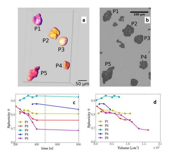
Figure 2: **a**: 3D rendering of the graphite particles P1-P5 after solidification. **b**: Room temperature SEI where particles P1 to P5 are pointed out. **c** & **d**: Sphericity of P1-P5 as a function of time and particle volume. The approximate end of graphite precipitation is indicated by a vertical line in a.
