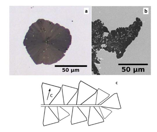
Figure 4: **a**: LOM image of spherical graphite particle with grains radiating from the centre and metallic inclusions between them. **b**: LOM image of protrusion from a graphite particle showing a dendrite-like structure. **c**: Schematic of a graphite dendrite with a stem from which grains grow along the "C" direction.
