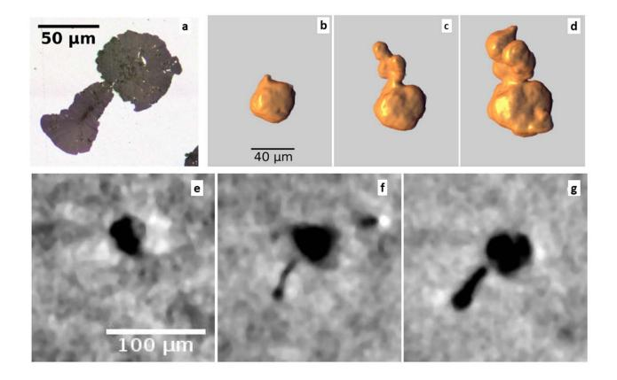
Figure 3: **a**: LOM image of graphite sphere with protrusion. **b-d**: 3D rendering of the particle in three stages of growth. **e-g**: 2D sections from the recorded X-Ray tomograms taken equivalent to the image in Figure 3a.
