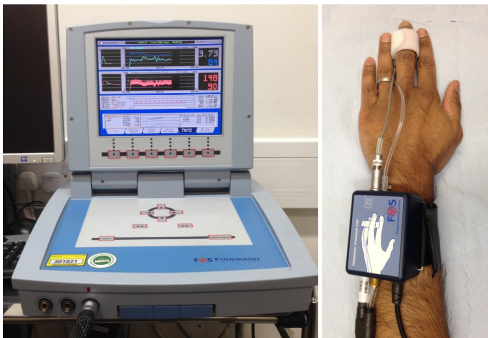
Figure 2-1: A Finometer was used for non-invasive beat-to-beat blood pressure measurements
