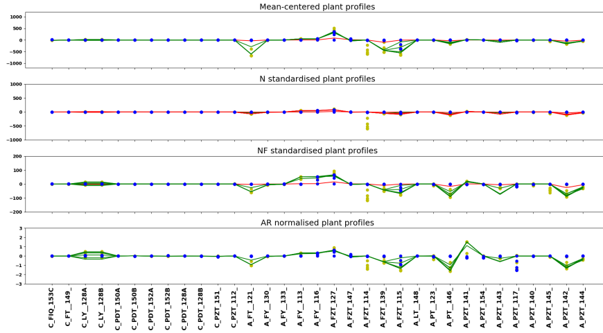
Fig. 4. Training plant profiles of class 2 (yellow points) and class 4 (blue points) and test plant profiles of abnormal situation A of class 2. The green lines are the test plant profiles that are correctly classified. The red lines are the test plant profiles that are misclassified as class 4. The classification uses one plant profile per feature vector.
