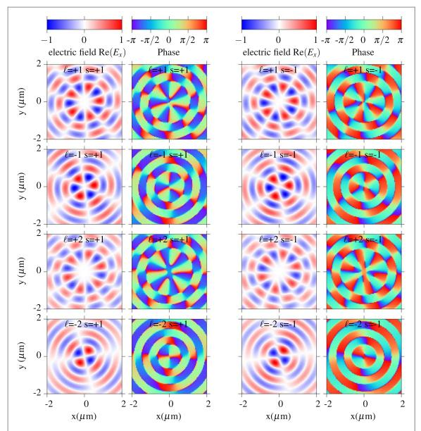
**Figure 3.** Electric field component  $Re(E_x)$  and phase of the scattered electric field of an Archimedean spiral with m=4 elements for OAM light excitation with  $\ell=\pm 1, \pm 2$  and  $s=\pm 1$ .
