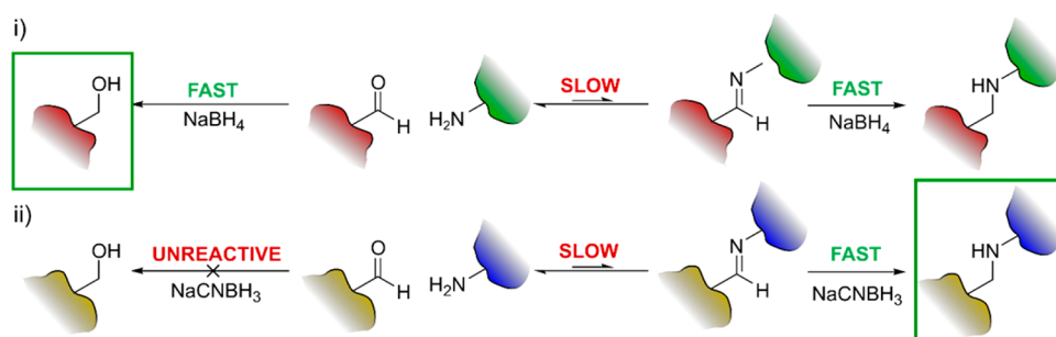
Figure 4. Imine formation is the rate-limiting step during reductive amination. Sodium borohydride is able to reduce the aldehydes which dominate and therefore fails to generate the desired conjugate. In contrast, sodium cyanoborohydride selectively reduces imines, leading to the formation of stable amine-conjugates.
