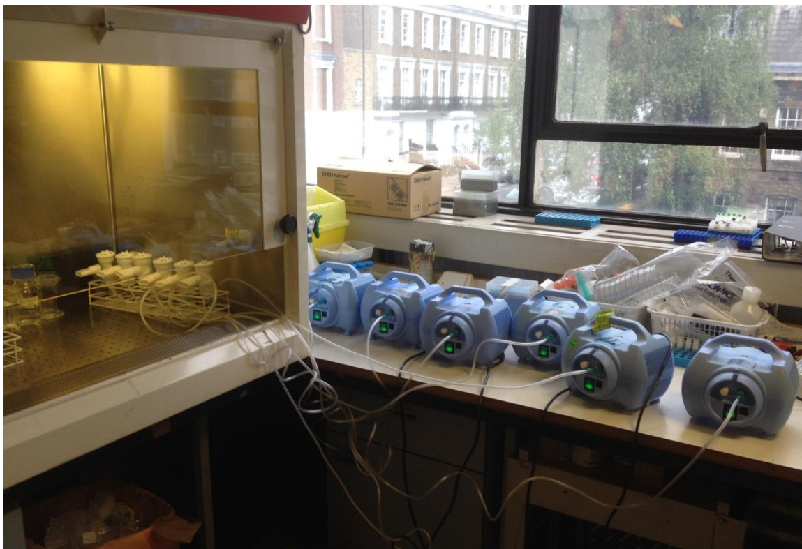
Figure 13.1.2: Experimental nebuliser set-up. Six compressors running in parallel, attached to AeroEclipse II nebulisers within biological safety cabinet. Compressors were stopped after 5, 10 and 15 minutes and 0.5ml aliquots of phage removed from the nebulisation chambers. These aliquots were subsequently analysed to establish remaining phage titres/ml and efficacy against PAO1.
