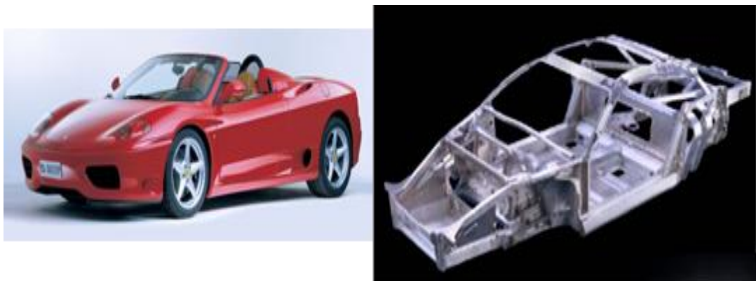
Figure 2-1 Profile based frame structure of the Ferrari F360 Modena (Kleiner et al., 2003; Kleiner et al., 2006; Jeswiet et al., 2008).
