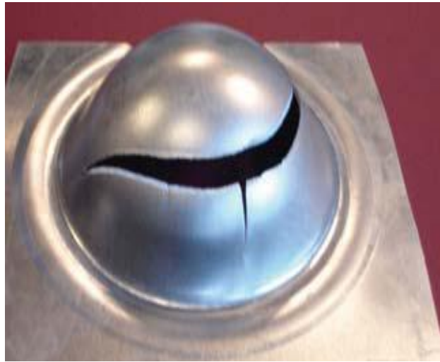
Figure 1-4 Low formability of cold forming T4 Al-alloy in a hemispherical punch test (Foster, 2008).
