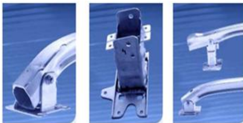
Figure 2-2 Aluminium extrusions in bumper beams and crash boxes (ArcelorMittal, 2008).
