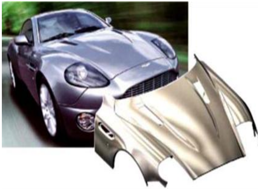
Figure 2-5 Superplastic formed aluminium sheets (Jeswiet et al., 2008).
