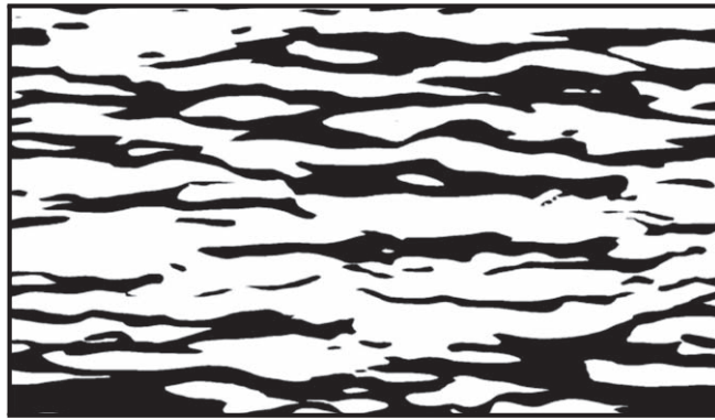
Figure 1. Near-wall streaks in a wall-parallel plane. Black areas correspond to regions of low velocity.
