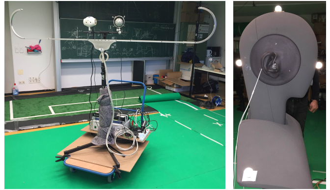
Figure 1. Recording environment and used microphone arrays with markers.
