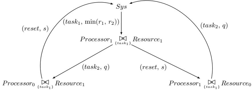
**Fig. 2.** Underlying CTMC of the PEPA model of Fig. 1
