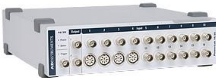
Figure 2.6: Appearance of the latest PowerLab
