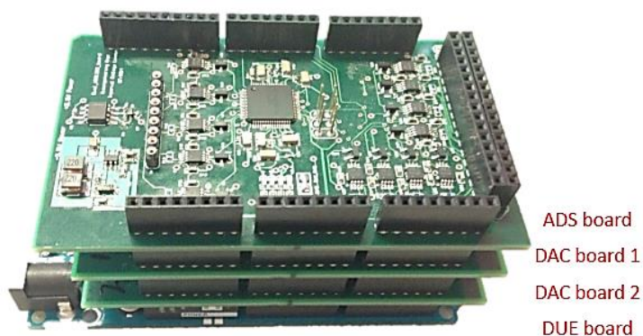
Figure 8.16: Stackable 16-channel voltage recording system
