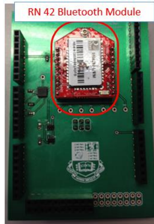
Figure 8.13: BT layer and relevant component arrangement
