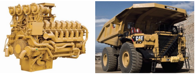
Figure 11. Caterpillar C175-16 engine (left) used in the Caterpillar 793 Mining Truck (right)
