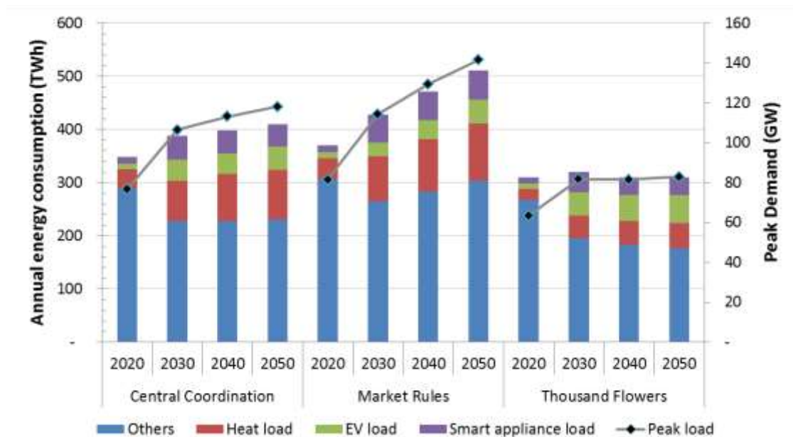
Fig. 2. Annual electricity demand and peak demand for different pathways which demonstrate the asymmetrical increase in the annual energy consumption and peak demand from 2020 to 2050
