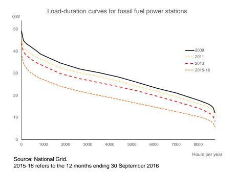
Figure 1: Load-duration curves for output from fossil fuel power stations
