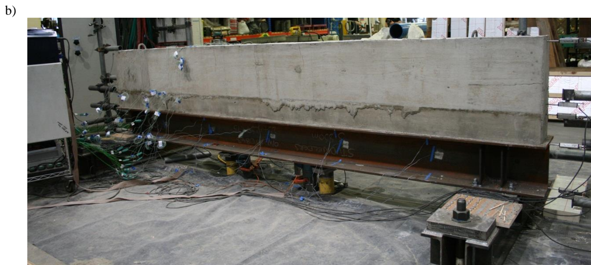
Figure 1: The experimental wall setup: a) elevation and transverse section of a 500 mm high wall (E-W3); and b) view of the experimental setup (All dimensions are in mm)
