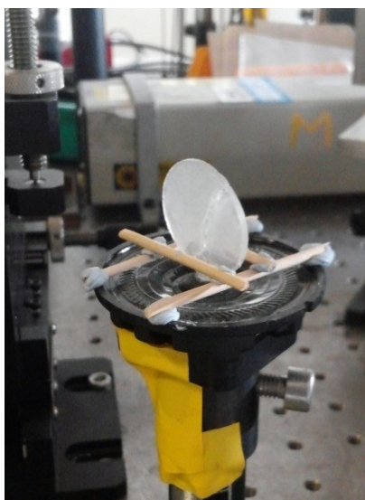
Figure 3-9. Photo of the diffuser implementation on a loudspeaker (left) and diagram showing diffuser and loudspeaker cone movement (right). When the loudspeaker is on, being driven a fixed frequency (usually 50-100Hz), the diffuser bounces about on the loudspeaker diaphragm. The diffuser is also allowed to pivot slightly. This motion is able to randomise the part of the diffuser the light passes through, giving a uniform time-averaged illumination and removing spatial coherence.
