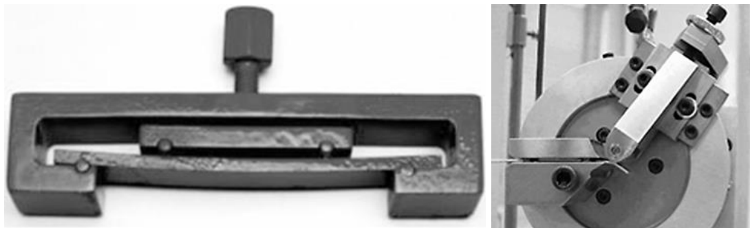
Figure 17. Left: A four-point bending SSC test jigs (Caltech Engineering Services, 2012). Right: A cantilever bend test to examine the formability of aluminium (McMaster University, 2007).
