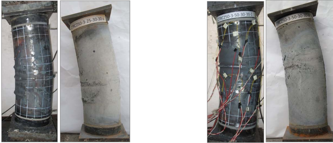
Fig.3 Typical failure modes of specimens (C30): (a) e=25\text{mm} ; and (b) e=50\text{mm} .
