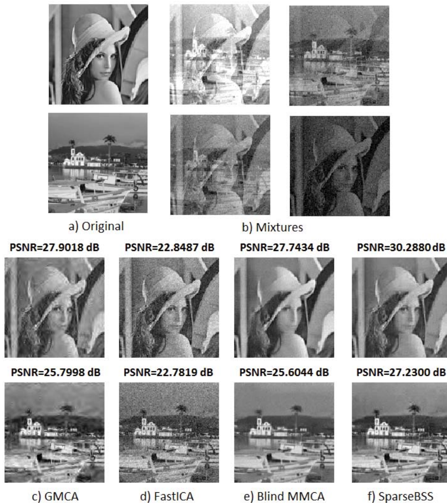
Figure 3.3: Two classic images, Lena and Boat were selected as the source images, which are shown in (a). The mixtures are shown in (b). The separation results are shown in (c)-(f). We compared SparseBSS with other benchmark algorithms: FastICA [57], GMCA [15] and BMMCA [1]. We set the overlap percentage equal to 50% for both BMMCA and SparseBSS. The recovered source images by the SparseBSS tend to be less blurred as compared to the other three algorithms.
